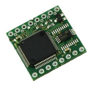
Elatec's Nano Module Multi125 LV is designed for integration into machines, handheld computer or any other device. The focus is set especially on size, price and flexibility.
